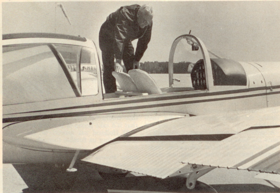
The French plane with 8° of flaps extended as Al Holland prepares to enter cockpit. Note how Fowler flaps increase wing area by nine square feet as they roll back six inches.
